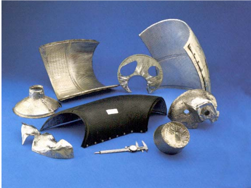
Various Aircraft Turbine Engine Bleed Air Ducts and Heatshields
